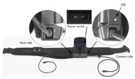
The arrows beside the cable connectors indicates that the round side of the IEEE 1394 connector should be facing this direction.
