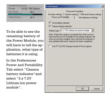
The power meter is updated whenever an image is captured so to get an exact reading you have to make a capture.
